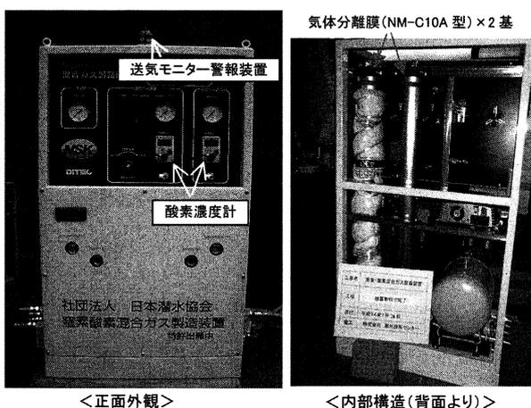
Fig.8 Overview of the oxygen enriched air generation system
